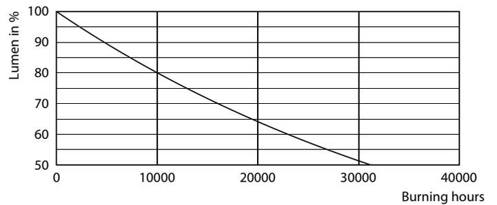
Lumen Maintenance Diagram - ESS LEDBulb 12-100W E27 6500K 1PF/6 MX
